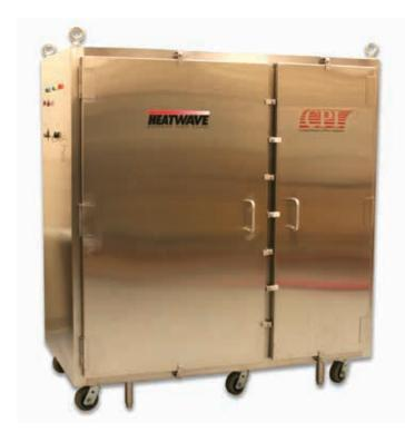
This integrated industrial microwave power system uses a CPI VKS-7960A klystron, designed for industrial service, as the energy source. By using the high-efficiency, 2.45-GHz, 60 kW CW klystron in combination with modern control and power supply technology, CPI is able to furnish a compact, userfriendly, cost-effective industrial system.
